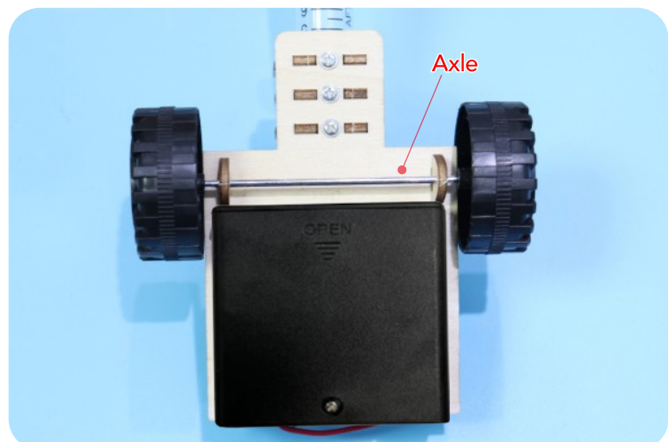
Step 10 - Pass the Axle through the holes of the two No. 5 plates, then install the two wheels on both ends of the axle.
